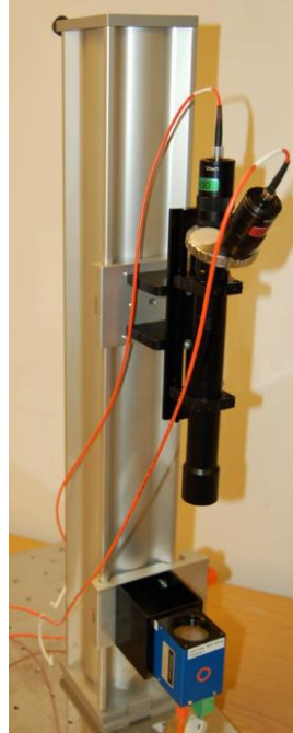
Figure 5: Shack-Hartmann sensor with collimated light source
