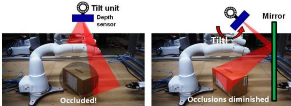
The concept of our tilt-based reflection sensing system. Credit: Yoshioka et al.
