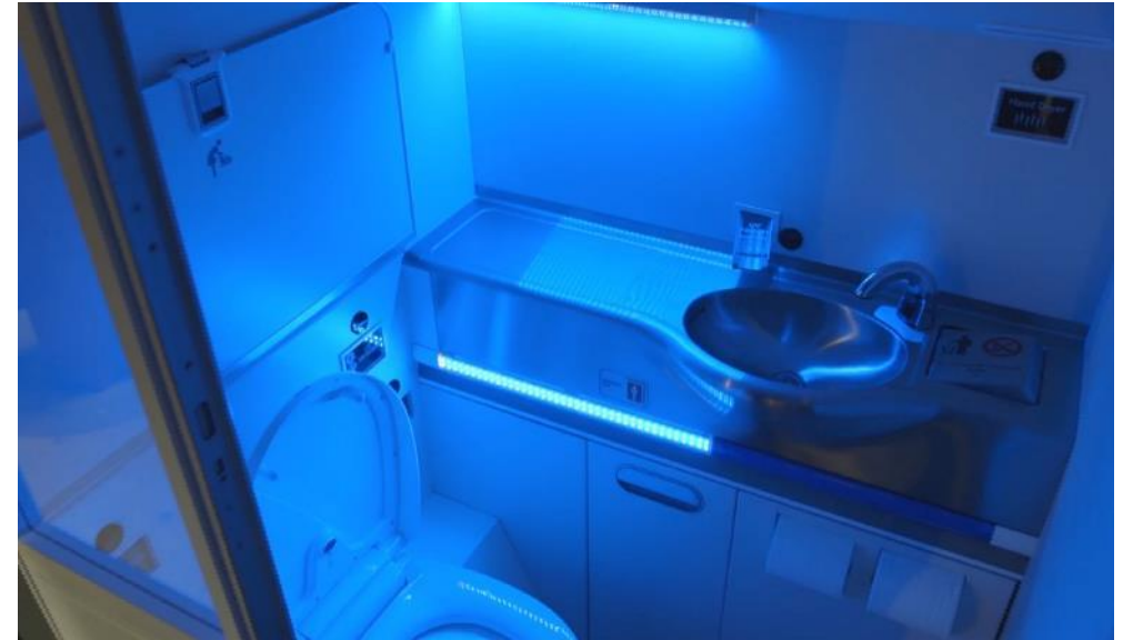
Boeing's self-cleaning lavatory zaps germs with UV light
