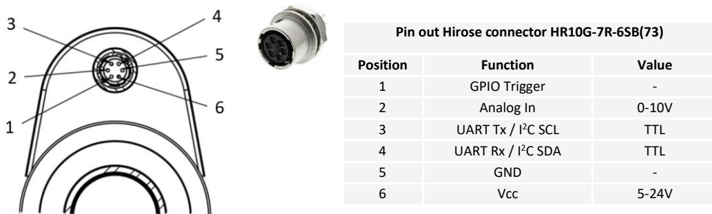
Figure 5: Electrical connections of lens models with embedded controller ECC-1C featuring (female) Hirose connector.
