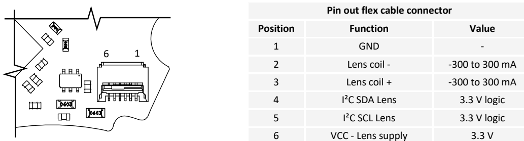
Figure 4: Electrical connections of flex cable connector.
